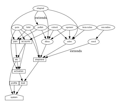
At the bottom, we see the *system service*, which produces the directory containing everything to run and boot the system, as returned by the **guix system build** command. See Section 12.18.3 [Service Reference], page 563, to learn about the other service types shown here. See [system-extension-graph], page 553, for information on how to generate this representation for a particular operating system definition.
