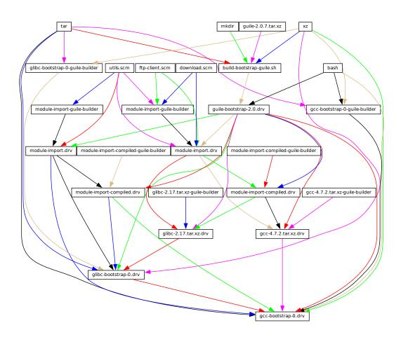
The figure above shows the very beginning of the dependency graph of the distribution, corresponding to the package definitions of the (gnu packages bootstrap) module. A similar figure can be generated with guix graph (see Section 10.10 [Invoking guix graph], page 201), along the lines of:
