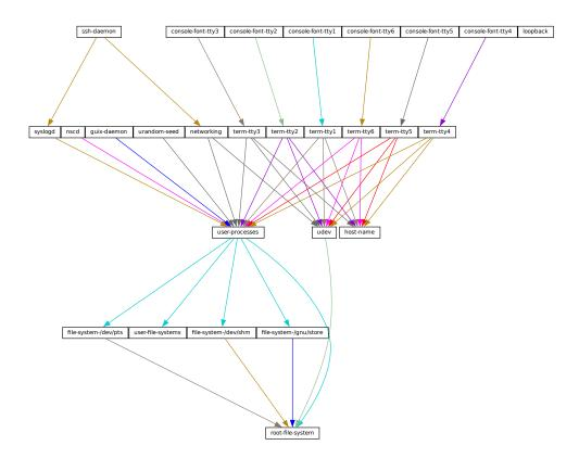
You can actually generate such a graph for any operating system definition using the guix system shepherd-graph command (see [system-shepherd-graph], page 554).
